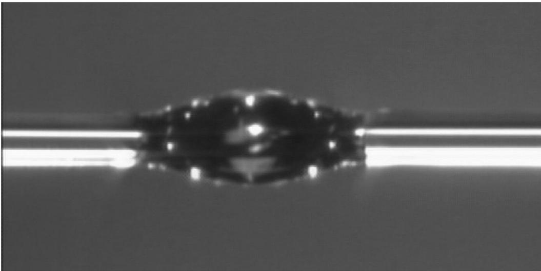
Fig. 2. Sideview of an optical coupling structure. The diameter of the fiber is  $125\ \mu\text{m}$  and the distance between the two fiber end is about 0.5mm.
