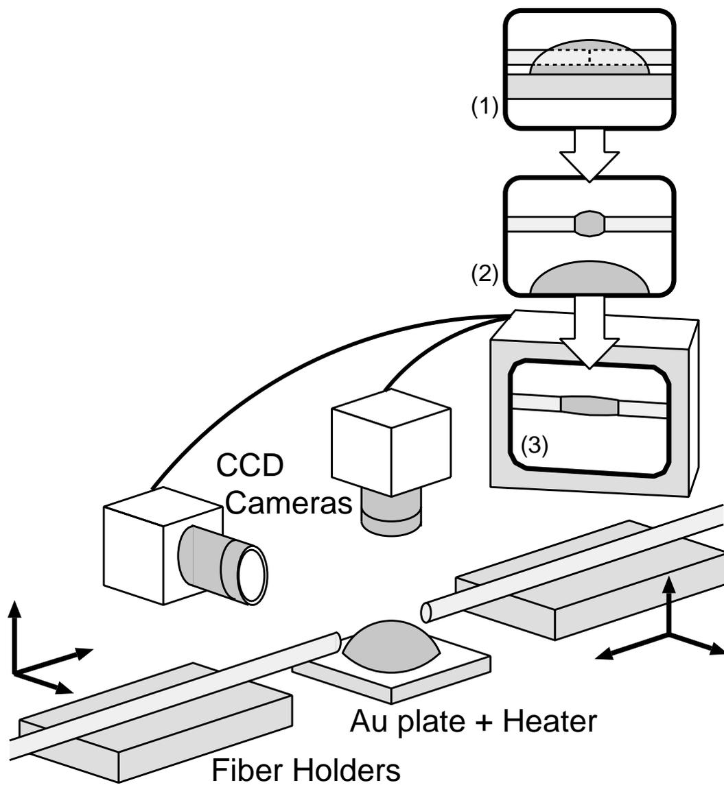
Fig. 1. Illustration showing an experimental setup and a procedure to make an optical coupling structure(see text).
