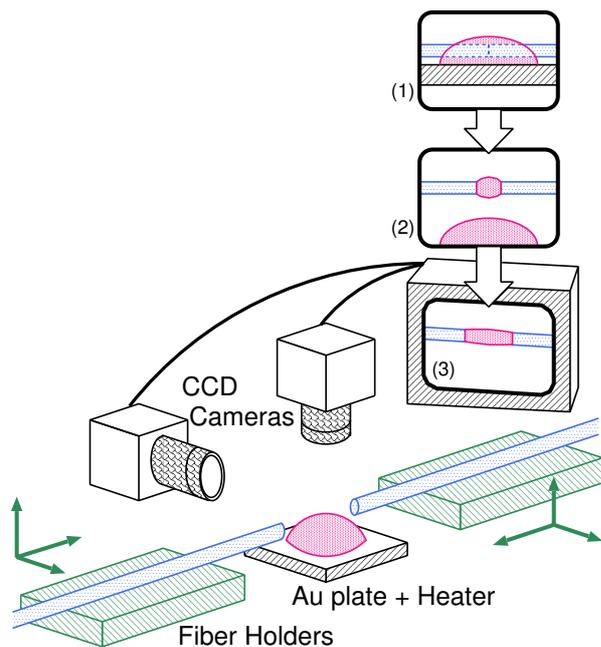
Fig. 2: Fabrication apparatus of splicing optical fibers via low-melting glass.
