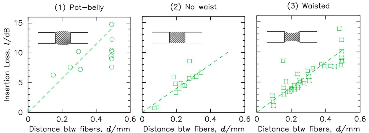
Fig. 5: Insertion loss values for spliced fibers via  $\text{TeO}_2$  glass as a function of distance between the fibers,  $d$ , classified into three groups according to the shape of inserted glass, (1) pot-belly, (2) no waist, and (3) waisted. Dashed lines are drawn by least square approximation, whose slopes are 28, 21 and 20 dB/mm, respectively.
