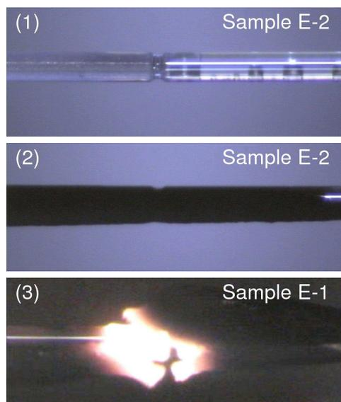
Fig. 1: Photographs of (1) a 50- $\mu\text{m}$ -thick  $\text{TeO}_2$  glass layer inserted in a silica glass fiber circuit, (2) carbon-coated spliced region, and (3) light-induced breakdown of this structure. The diameter of the fiber is 125 $\mu\text{m}$ . The light source is connected to the right side.
