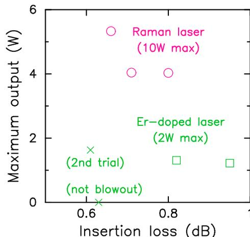
Fig. 3: Maximum output values from the present optical fuses vs. their insertion loss for 1.3 $\mu$ m.
