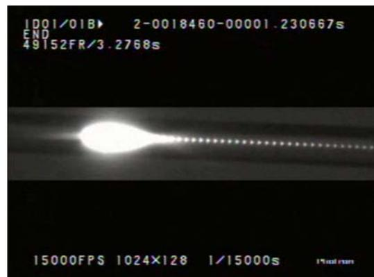
Figure 4: The first captured image of fiber fuse propagation. The image is saturated in spite of the exposure time of 1/15000 second.
