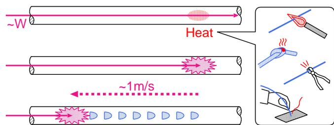
Figure 3: Fiber fuse ignition, propagation and periodic void formation.
