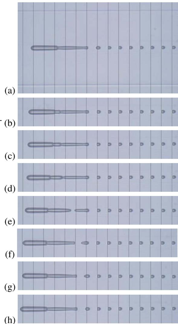
Figure 6: A series of optical micrographs showing the damage generated by 5.0 W laser light. The interval of the vertical lines is  $17.8 \mu\text{m}$ . The micrograph at the bottom is the same as that at the top, shifted  $17.8 \mu\text{m}$  to the left.
