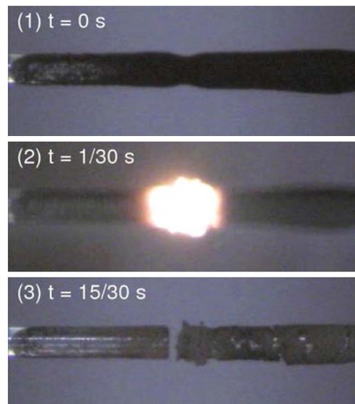
Figure 1: Breakdown of optical fuse. The outer diameter of the optical fiber is 125  $\mu\text{m}$ .
