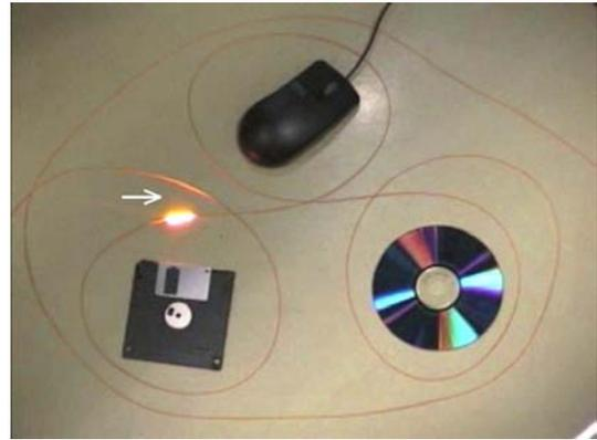
Figure 2: Macroscopic view of fiber fuse propagation through a single-mode silica fiber pumped by a 9.0 W and 1.48  $\mu\text{m}$  laser light.
