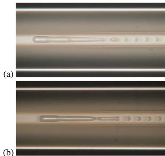
Figure 5: Optical micrographs of fused damage generated by a laser light of 1480 nm, 9.0 W. The images are distorted due to the absence of matching oil. The distance between the two horizontal white lines corresponds to the diameter of the optical fiber, 125 μm.
