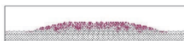
Charge distribution of Ge cluster on Si(001) surface (23,737 atoms) around Fermi level
