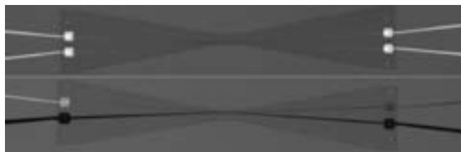
Figure 2: Parallel electrodes before the deposition of polyaniline (top) and after (bottom).
