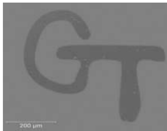
Figure 4: Bioconjugated and photobleached SiO 2 substrate.
