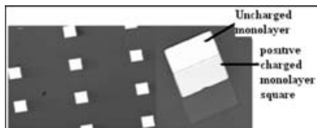
Figure 3: Patterned monolayer substrate (on left). Double patterned partially charged square (on right).
