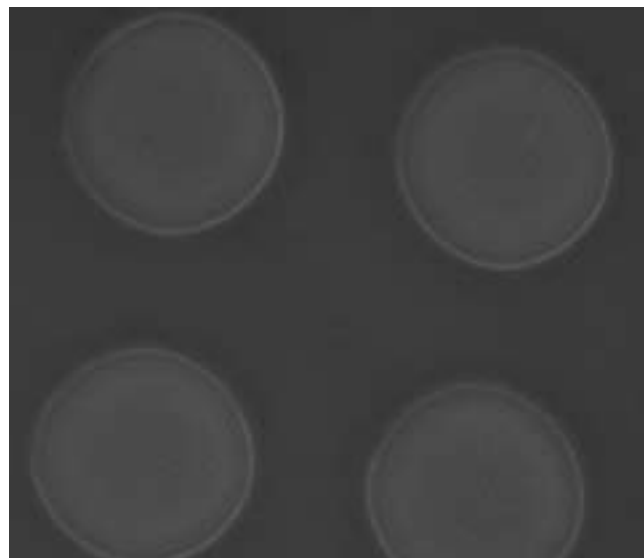
Figure 1: 10 \mu\text{m} hole pattern in the substrate.
