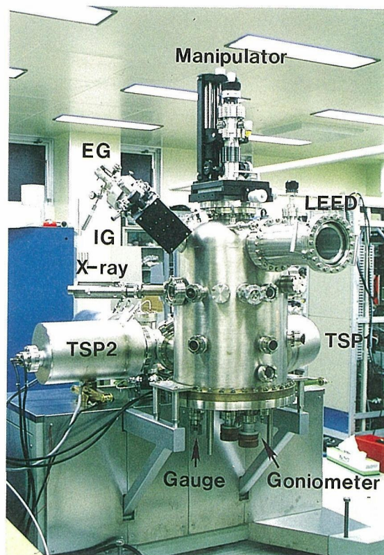
Fig. 3 Photograph of a newly developed HR-ARES system.
