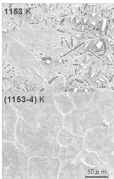
Fig. 10 SEM images of the oxide layer at the oxide/silver interface of the tape quenched from 1153 K. The temperature gradient was 200 K/m. The upper figure shows the higher-temperature region, and the lower one shows the lower-temperature region
