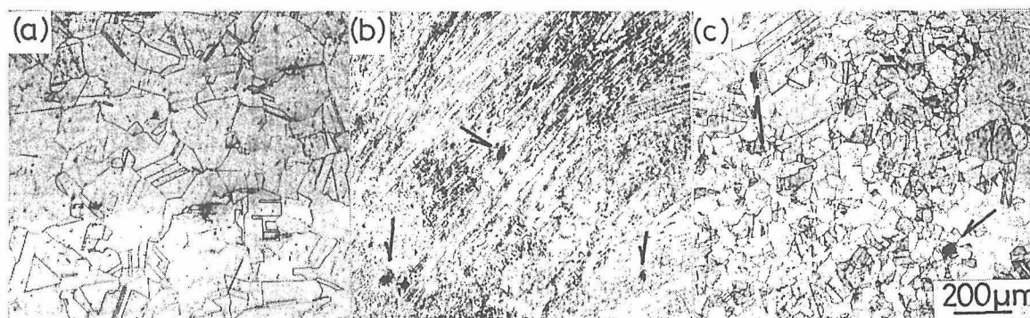
(a) Base metal (b) Weld metal (c) Recrystallized weld metal containing micro-defects. The micro-defects in (b) and (c) are arrowed.
