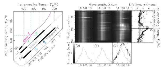
Fig. 3: Annealing condition of the sample libraries and appearance of the annealed glass segments inside. (0) with no annealing treatment for reference. (1) with 1st annealing for 5min only. (2) with two successive heat treatments, each for 5min. Thick black line: completely transparent segment, thin black line: white, and medium gray line: opaque(see text).  $A_n$  and  $B_n$  indicate specific glass segments. These notations are also used in Fig. 4.
