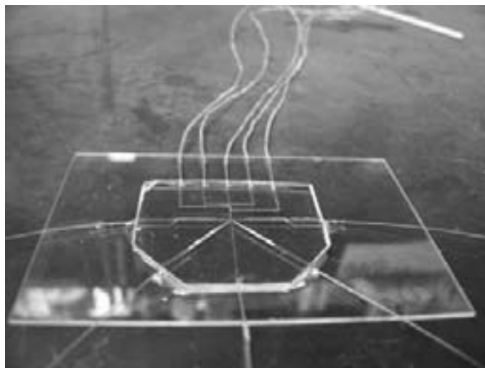
Figure 1: Assembled flow cell with channels that have a cross section of 100\text{ }\mu\text{m} by 100\text{ }\mu\text{m} .
