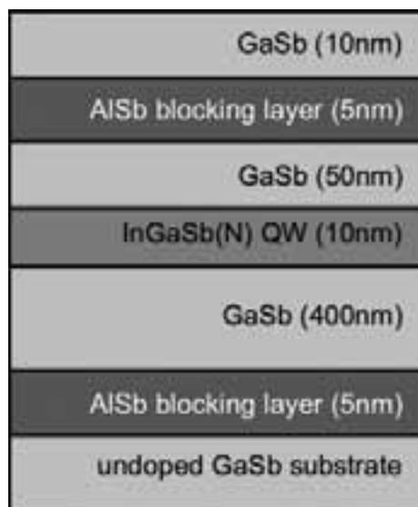
Figure 1: Sample structure used for annealing studies.
