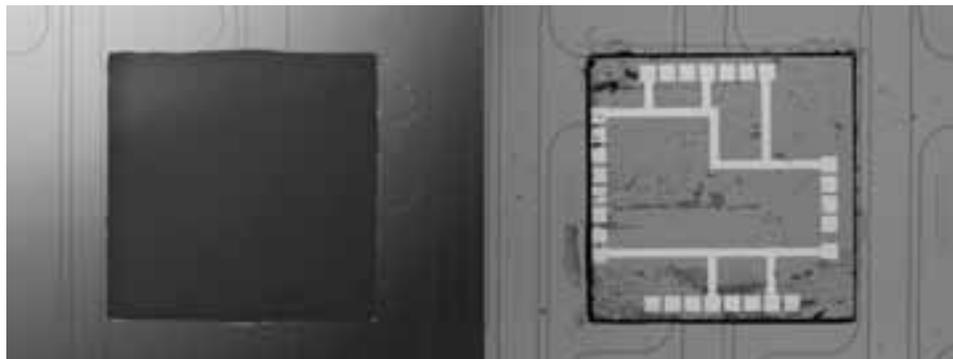
Figure 2: Vacant through-substrate cavity (left) and integrated RLC circuit die (right).
