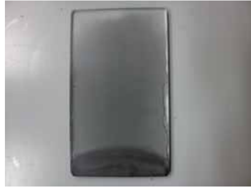
Fig.5 Horizontal alignment of CNTs in TiO 2 . There is no crack and aggregation. The thickness of film was approximately 100-150nm.
