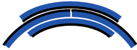
Fig. 2a. Three-layers joint: the upper tape is soldered with the YBCO layer (black) facing the jointed tapes, while the bottom tape is soldered with the hastelloy substrate (blue) facing the jointed tapes.
