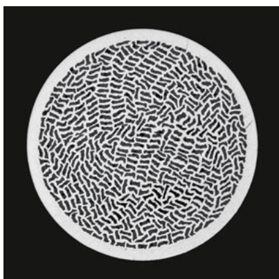
Fig.1. Cross sectional view of the Bi-2212 wire having low silver ratio.
