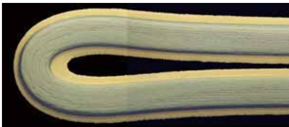
Fig. 3. 180 degree bent test for F3 strand.
