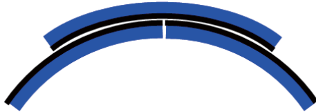
Fig. 2b. Two-layers joint: only the upper tape is used to joint the tapes.
