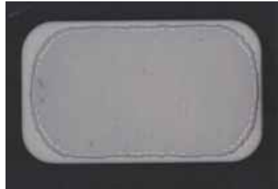
Fig.1 Cross-sectional view of the Nb 3 Sn wire used 17wt%Sn Bronze
