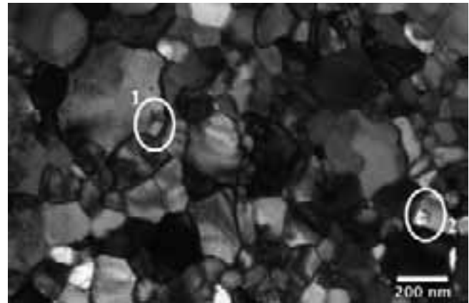
Figure 3: Dislocation pile-up observed in larger grains.
