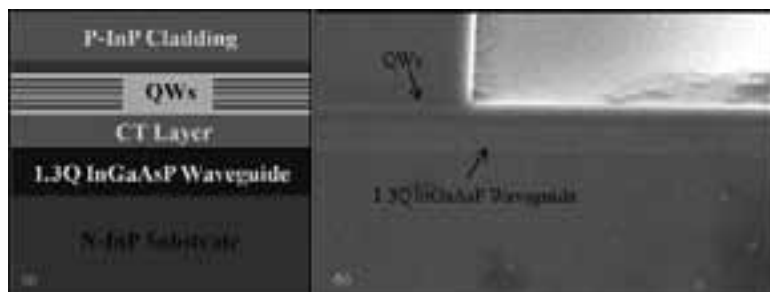
Figure 1: (a) Schematic of CTL epitaxial design, (b) SEM of fabricated 100 nm CTL design active region.
