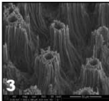
Figure 3: SiNWs that have self-densified into structures during a one hour etch.
