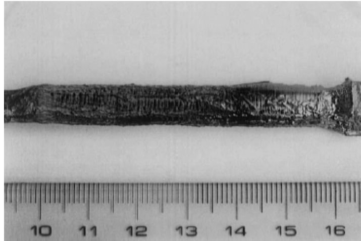
Fig. 2. A single crystal of \text{ScB}_{19+x}\text{Si}_y grown by the floating zone method.
