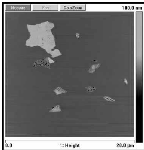
Figure 1: \text{Al}_2\text{O}_3 deposition on \text{MoS}_2 flakes with no treatment. The black regions are devoid of \text{Al}_2\text{O}_3 .
