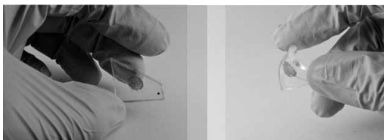
Figure 3: Silver nanoplates deposited onto the surface of PDMS. This is the first step towards flexible electrodes that utilize these plates.
