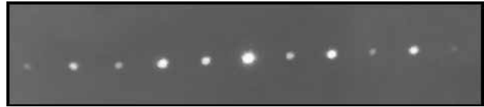
Figure 4: Pattern from a double grating shifted by one half of a period.
