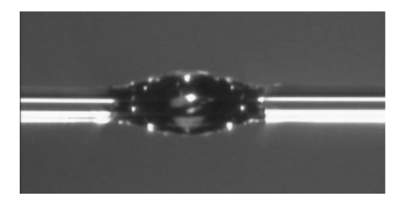
Fig. 2. Sideview of an optical coupling structure. The diameter of the fiber is 125  $\mu$ m and the distance between the two fiber end is about 0.5mm.
