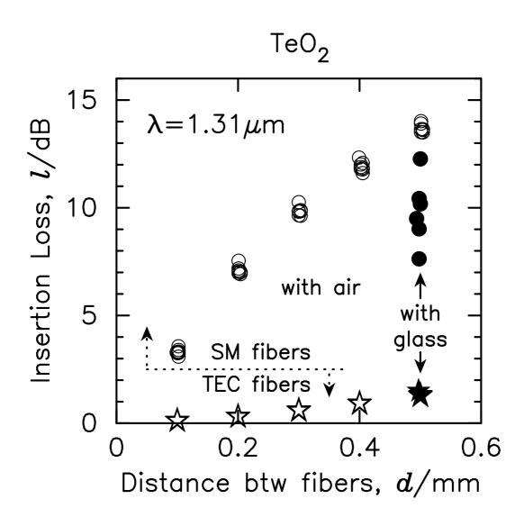
Fig. 3. Insertion loss vs. distance between the two fiber ends for the optical coupling structure (closed marks) and an empty fiber pair (open circles).
