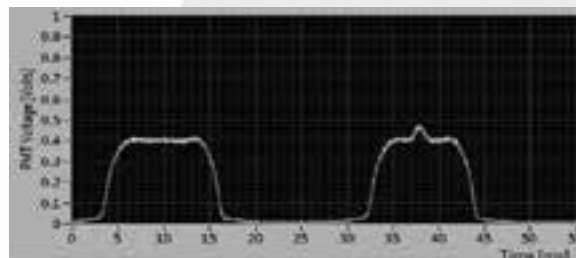
Figure 4: Time-trace snapshot of droplets detected using PMT. The plateaus indicate the fluorescein concentration in droplets, while the peak atop the second plateau indicates an apoptotic cell.
