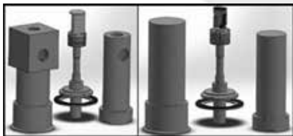
Figure 3: SolidWorks models of both versions of the new cryostat components, optical (left) and electrical (right).
