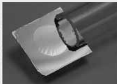
Figure 4: Optical imaging reveals no cracks in the suspended foil. (See full color version on page xxxvi.)
