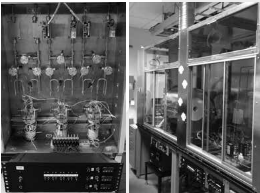
Figure 3, left: Finished MOCVD gas panel and switch box. Figure 4, right: Fully ventilated protective enclosure.
