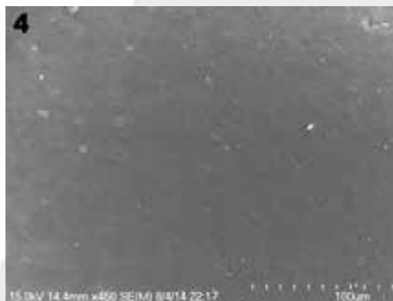
Figure 4: Sample 7/23-2. Amorphous film allows for even distribution of the dopant. Ethanol allows for fewer surface defects (e.g., pores, cracks, etc.).
