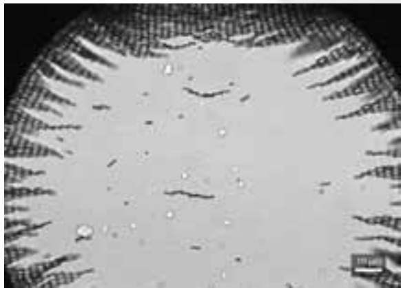
Figure 3: A 100 \mu\text{m} bulb region of the bulb-stem electrode during assembly.
