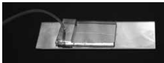
Figure 1: A PDMS flow chamber prototype for particle sorting using optical forces.
