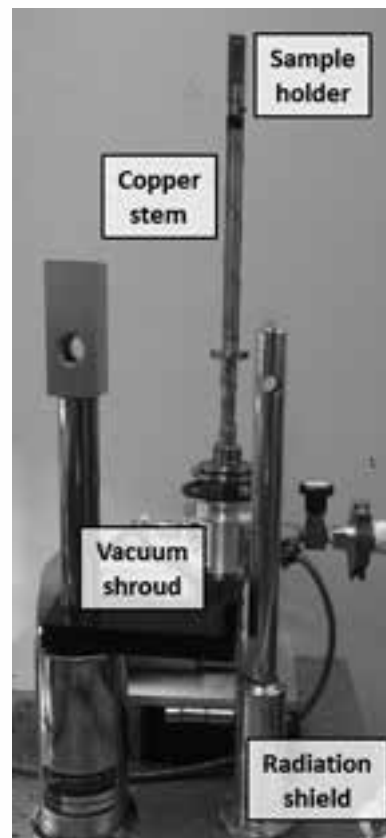
Figure 2: The former cryostat, disassembled. Labeled components were modified.
