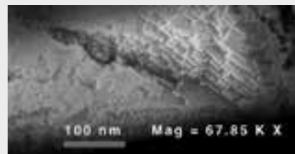
Figure 3: Infiltrated \text{SnO}_2 opal at a dose of 0.090 s of \text{TDMA}_{\text{Sn}} and 0.045 s of \text{H}_2\text{O} .
