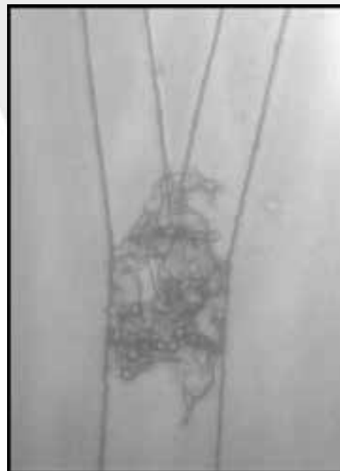
Figure 2, right: Dust clogging in the flow chamber at the fork.
