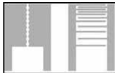
Figure 2: The two electrode designs: bulb-stem (left) and interdigitated (right).
