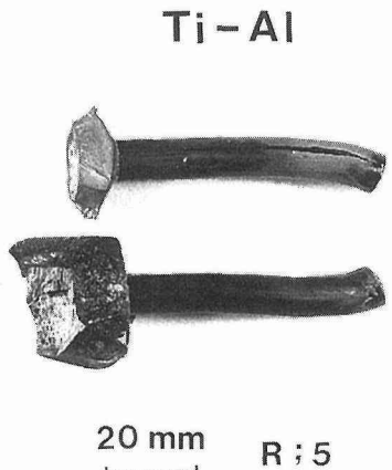
Fig. 22 Examples of extruded stoichiometric TiAl compound with the method shown in Fig. 21. Dies made of \text{Si}_3\text{N}_4 were used and TiAl billets were heated at about 1600 K.
