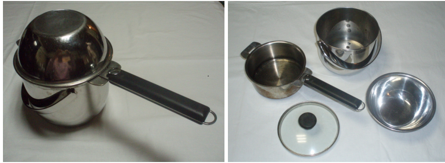
Figure 3: Handmade cooking apparatus for heat insulation comprising a milk pan (14 cm), an ice pail, a glass cover and a bowl.
