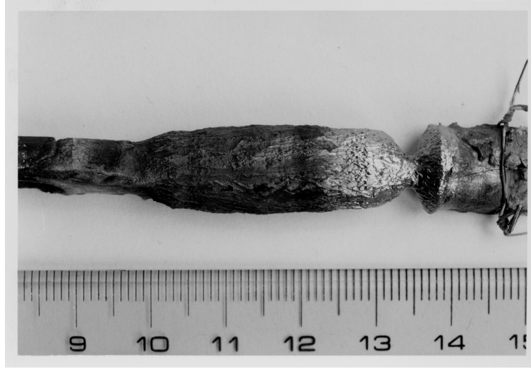
Figure 18. An example of \text{ScB}_{15}\text{C}_{0.8} crystal [20].
