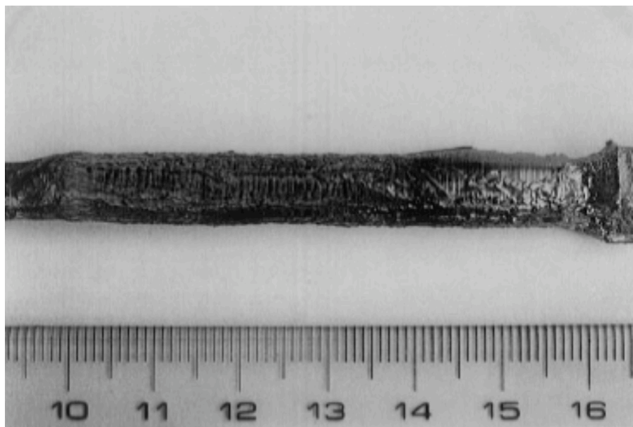
Figure 14. Single crystal of \text{ScB}_{19+x}\text{Si}_y [16].
